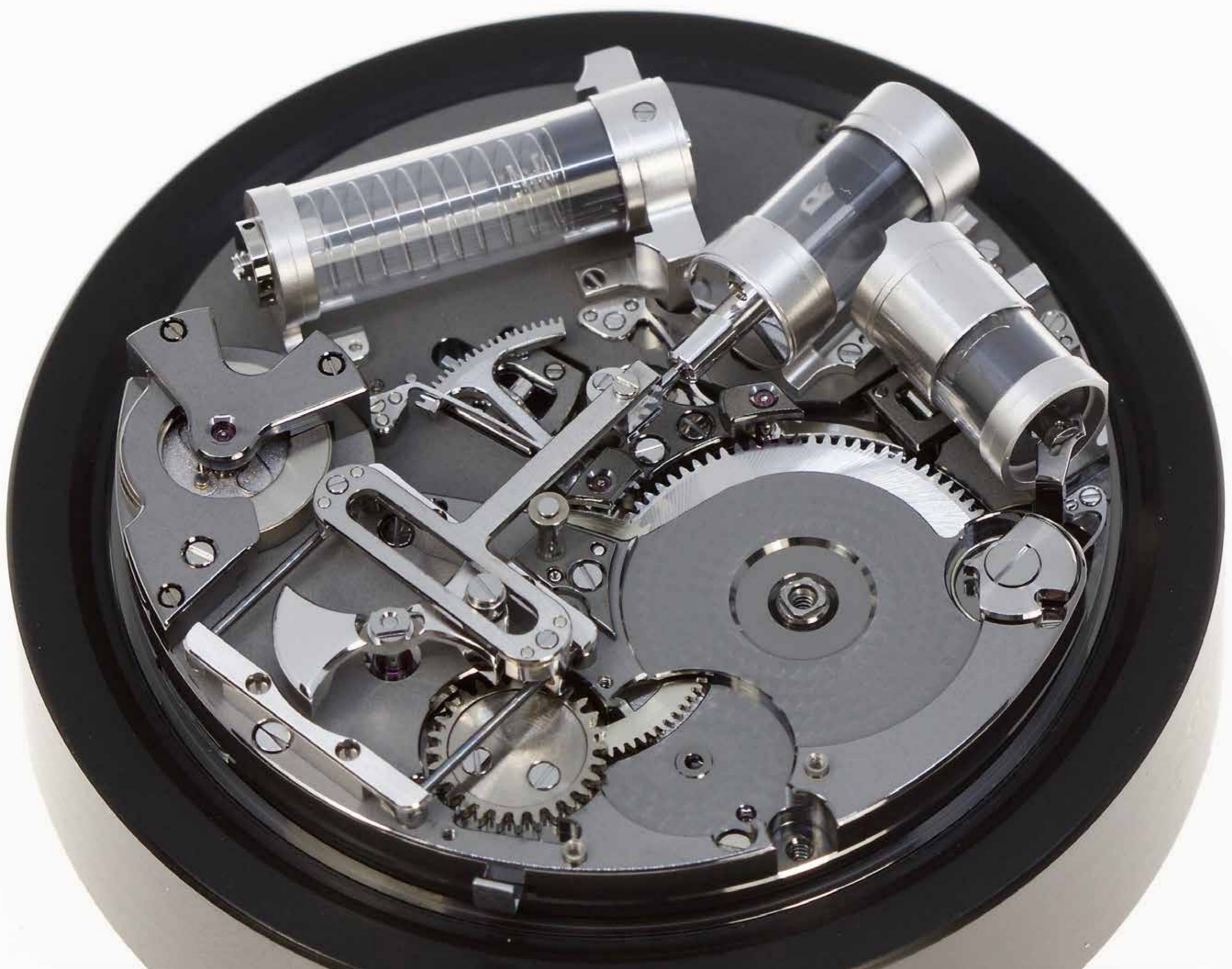
The ratchet wheel, and part of the winding mechanism removed.
